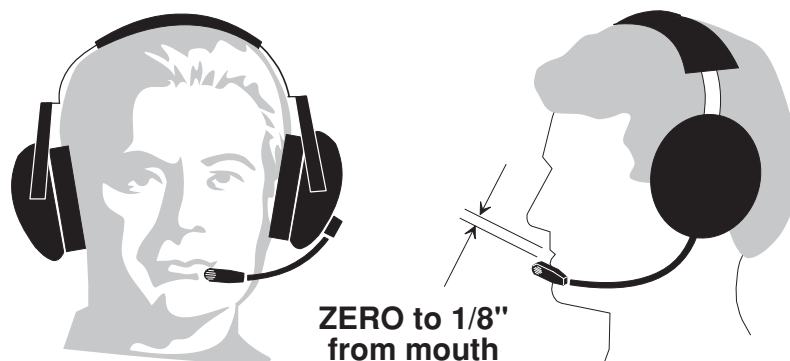
Figure 12 - Correct Positioning of Boom and Microphone
